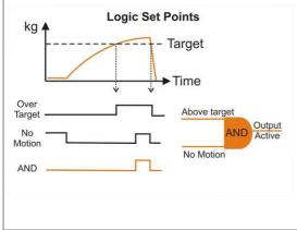
R400 Logic set points are based on the status of the inputs and the defined mask that is used to match IO1-IO24 for the logic set points.
